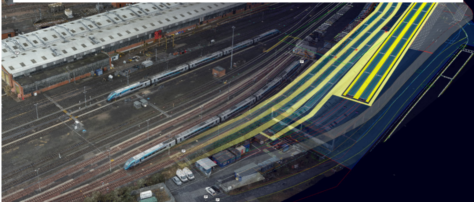
Above SLC's digital twin of the site created using a 3D pointcloud visualised overlaid with CAD designs.
